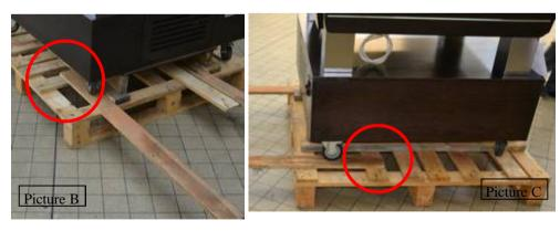
3. Place one of the four unloading planks under one of the castor. Push it until the first slat of the pallet (see red circles in pictures B and C)
