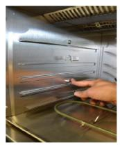
c) Assembly and removal of the bottom heating element
