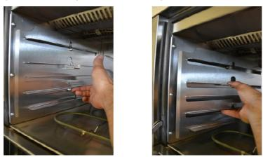
To replace the scales, place them on the 2 pins, press slightly and let slide down.
