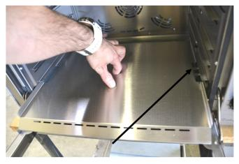
To replace the bottom heating element cover, proceed in the reverse order. Take care, place the bottom heating element cover in the right way
